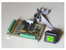
Ribbon Cable - The 18" ribbon cable allows easy to installation and removal if necessary. Plugs are provided at both ends. The driver board was designed to mount lower in the instrument panel for easy access to wiring.
