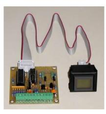
Ribbon Cable - The 18" ribbon cable allows easy to installation and removal if necessary. Plugs are provided at both ends. The driver board was designed to mount lower in the instrument panel for easy access to wiring.
