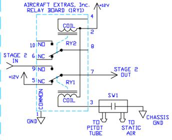
SW1 is an adjustable indicated airspeed switch. Its setpoint is screwdriver adjustable. The switch is closed above its airspeed setpoint. The output voltage of this stage is 12V when SW1 is open. When SW1 is closed, the output voltage of this stage is equal to the input voltage of this stage.
