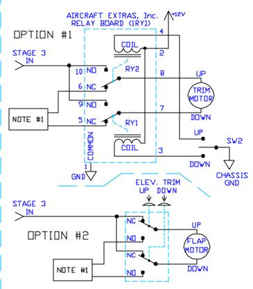
Use option #1 of this stage if you use a Single Pole, Double Throw, (DN)-DFF-(DN), momentary, 3 position switch for your elevator trim control. . Use option #2 if your elevator trim control switches can be wired as two independently actuated switches.
